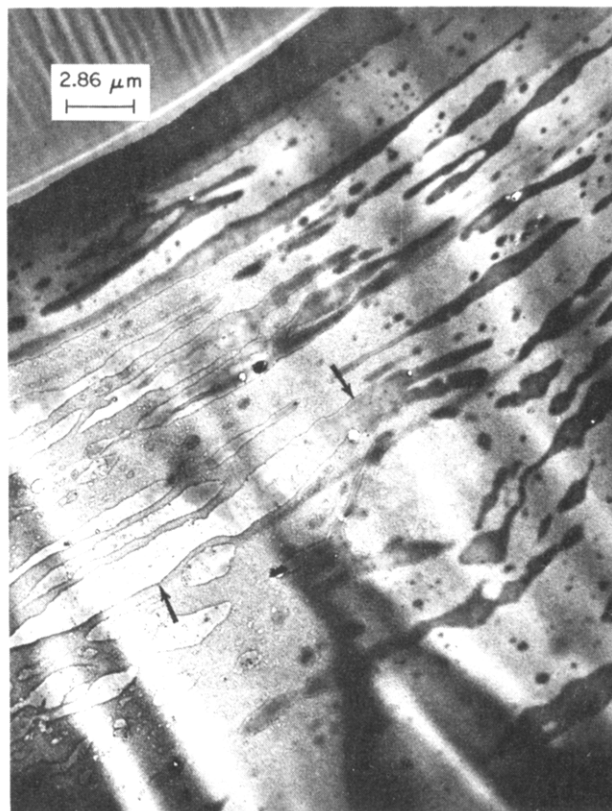
Figure 1. Cross-sectional micrograph of a pressed film of a 25% carboxylate/75% sulfonate blend of perfluorinated ionomers. The elongated regions (arrows) are the carboxylate phase.
